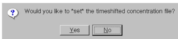
Answering "yes" will then associate the re-peaked, time-shifted concentration data to the  $I(t)$  vs.  $t$  SAXS dataset under analysis. This operation can be anyway performed at any time by selecting only a concentration chromatogram dataset, and pressing **Set**. The concentration chromatogram shown in this example is then cropped to have approximately the same frame number as the SAXS  $I(t)$  vs.  $t$  chromatograms.
