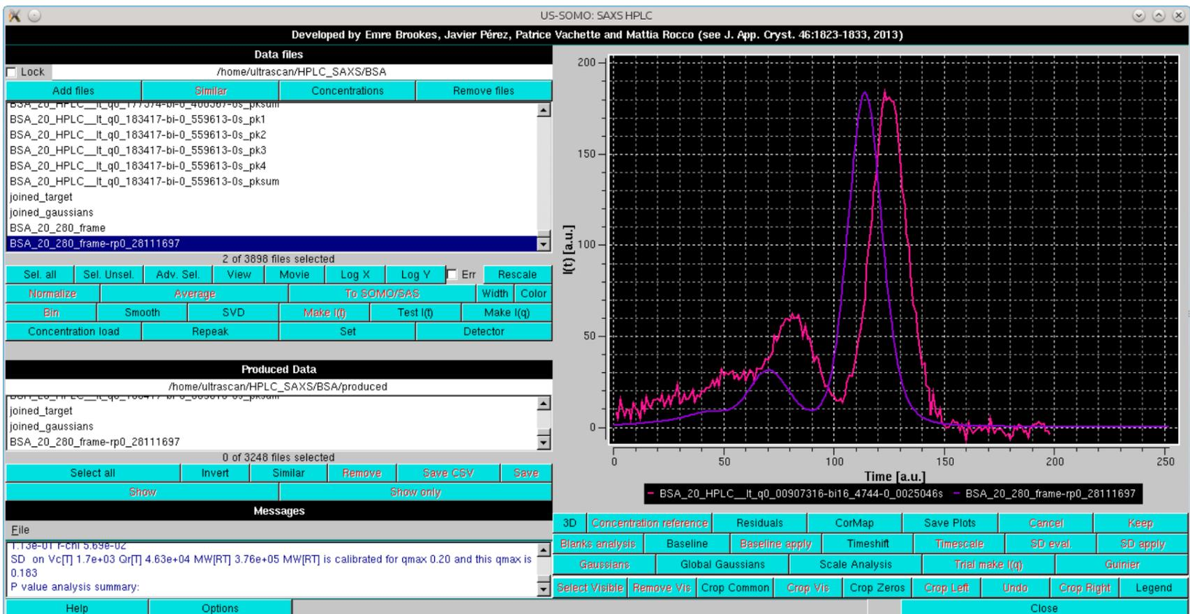
After re-peak, the concentration chromatogram usually must be time-shifted to align its peaks to the  $I(t)$  vs.  $t$  chromatograms using the **Timeshift** button.
