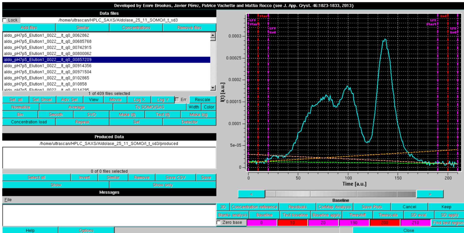
By clicking on each field, the corresponding line can be moved across the chromatogram using the *gray-shades bar-wheel* at the top of this panel or the "<" and ">" buttons placed at its sides. The actual baseline is shown as a green dashed line, while the two orange dashed lines show the trends of linear regression done on the regions delimited by the two couples of vertical magenta lines. Ideally, the orange lines should come as close as possible to the green line:
