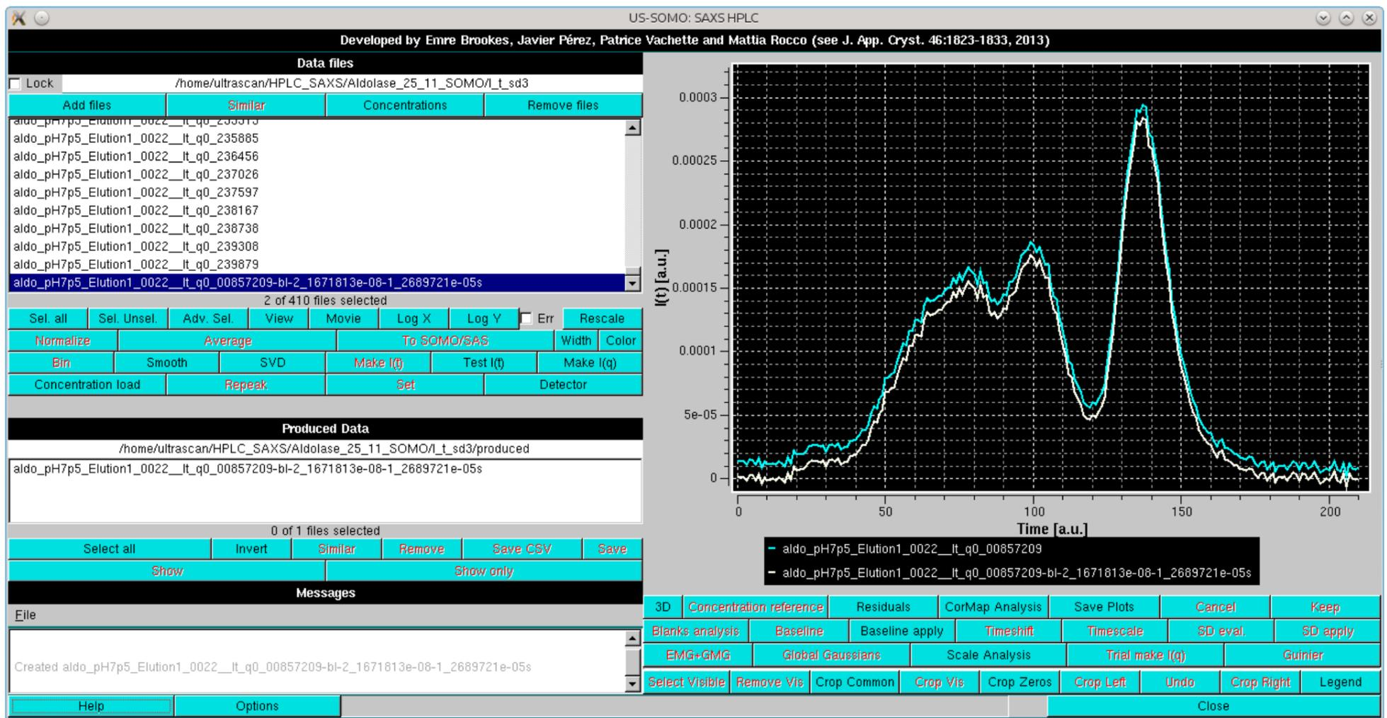
The baseline parameters thus set can be applied to all curves with concurrent subtraction of each baseline by selecting them all and then pressing again the **Baseline apply** button. A new set of data is generated, the initial and final points used in the linear baseline subtraction are added to the filename of the produced files, and two labels are added, "-bl" (=baseline linear) after the  $q$  value, and "-s" at the end of the filename, as shown in the **Data files** panel:
