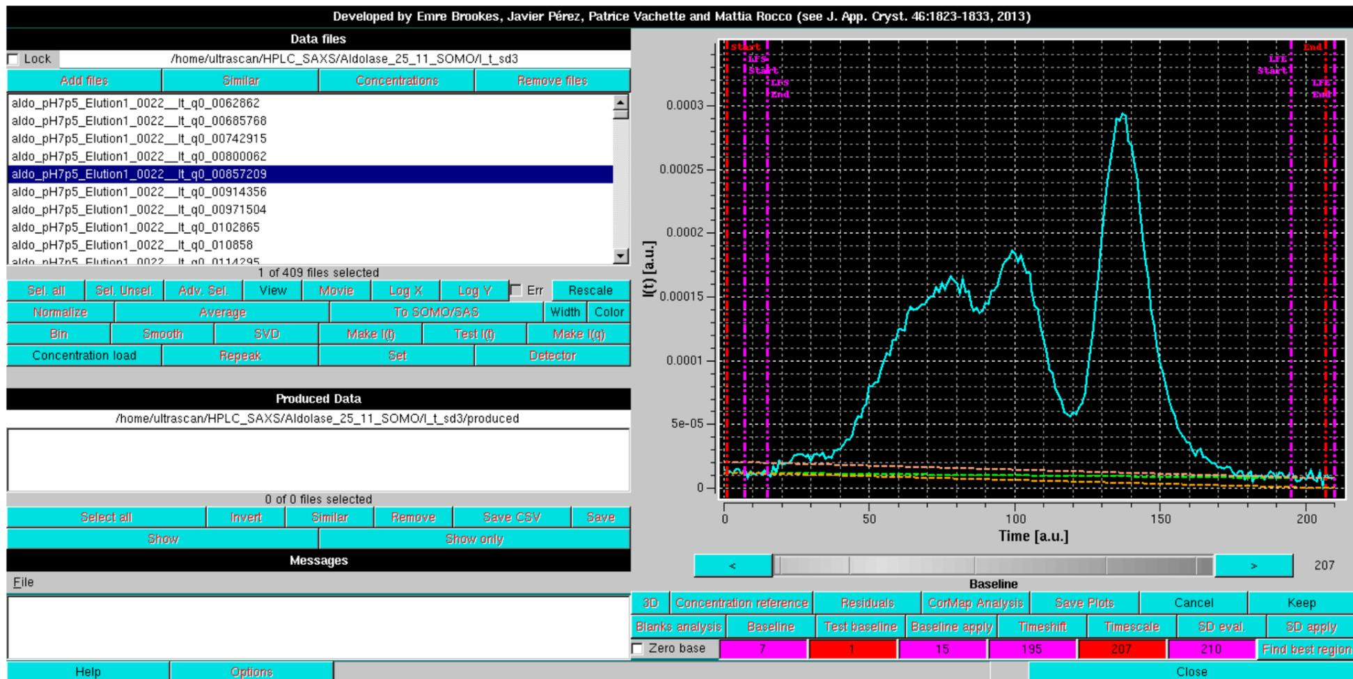
Pressing **Keep** once a reasonable baseline has been found will keep its parameters (initial and end points, slope) for further operations.
