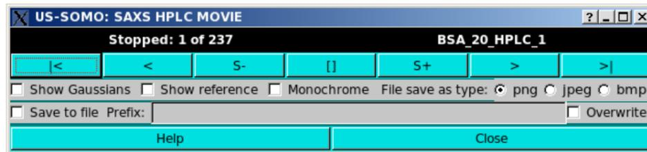
This utility allows to view in the main graphics window of the **US-SOMO HPLC-SAXS** module a series of data files in a movie-like manner, and to optionally save each frame as an image for real movie-making operations.
