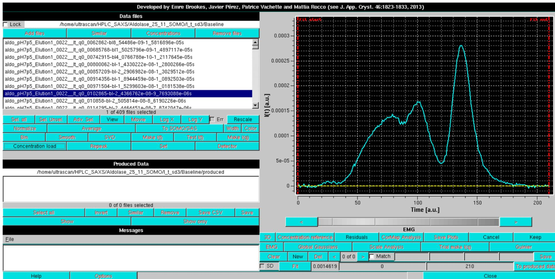
Since an *SVD* analysis (see [here](#)) on this dataset (not shown) indicated that four components were at least needed to describe it, four EMG Gaussians are initially positioned:
