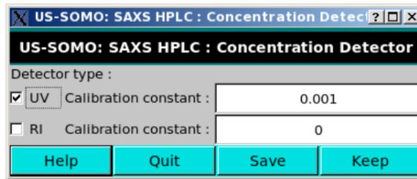
This utility will allow to select the type of detector and to enter its calibration constant. Two types of concentration detector are currently supported, UV and refractive index. The used detector can be selected by clicking on either of the two *Detector type*: checkboxes and entering the calibration constant converting their signal in the proper units (absorbance or dn/dc) in the fields to their right:
