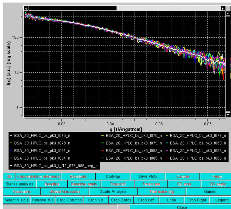
In the latter, an average curve (obtained by pressing the *Average* button) is also superimposed. Such re-generated  $I(q)$  vs.  $q$  data can be directly exported in the main US-SOMO SAS module for further
