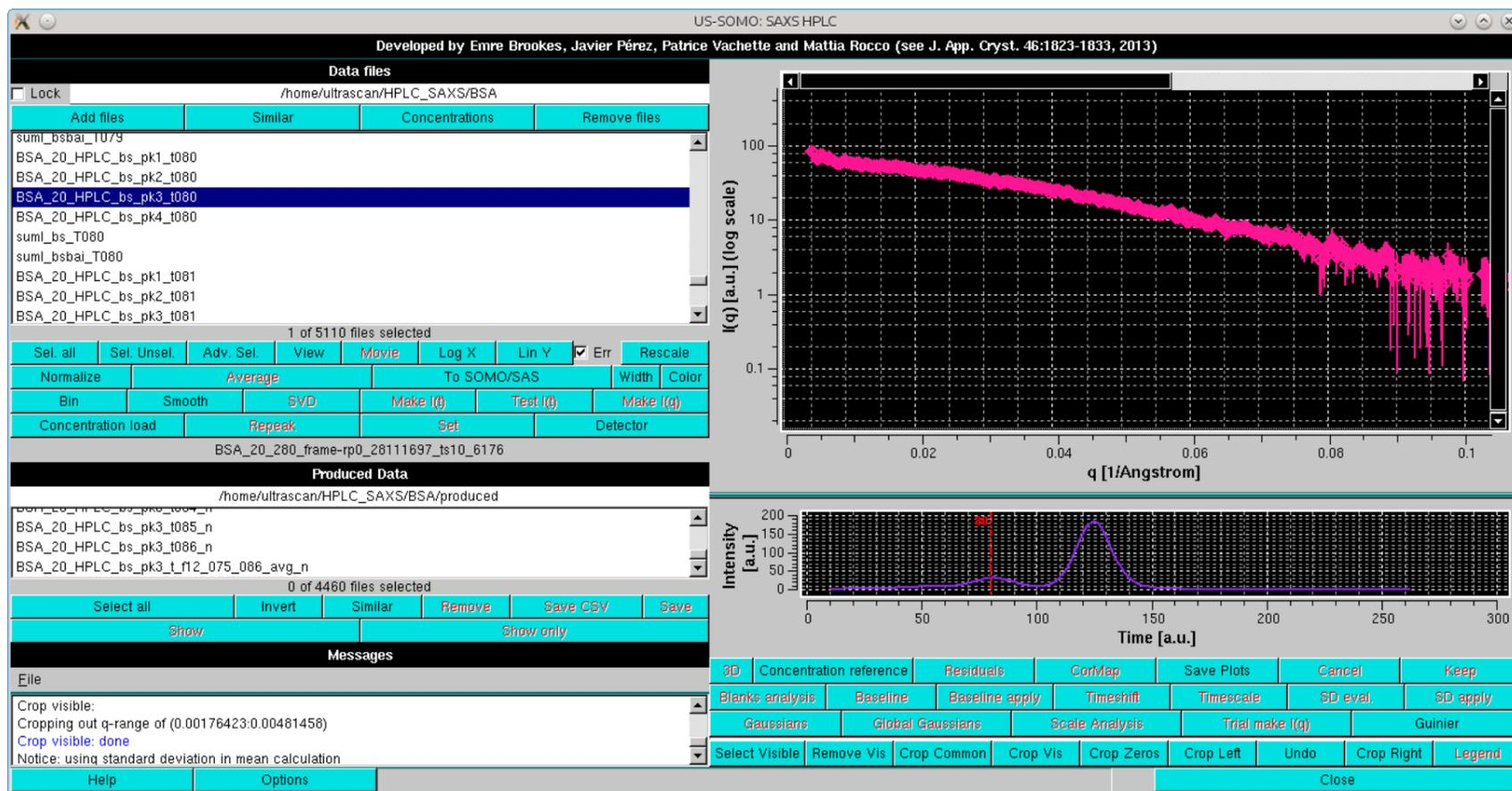
In the example shown above, the  $I(q)$  vs.  $q$  data for the decomposed peak #3 frame #80 are shown with their associated errors, and below it the position of this dataset is shown by the vertical red line on the associated concentration chromatogram. Each time a different chromatogram is selected, its position will be mapped on the concentration plot. Pressing the **Concentration reference** button again will make this additional plot disappear.
