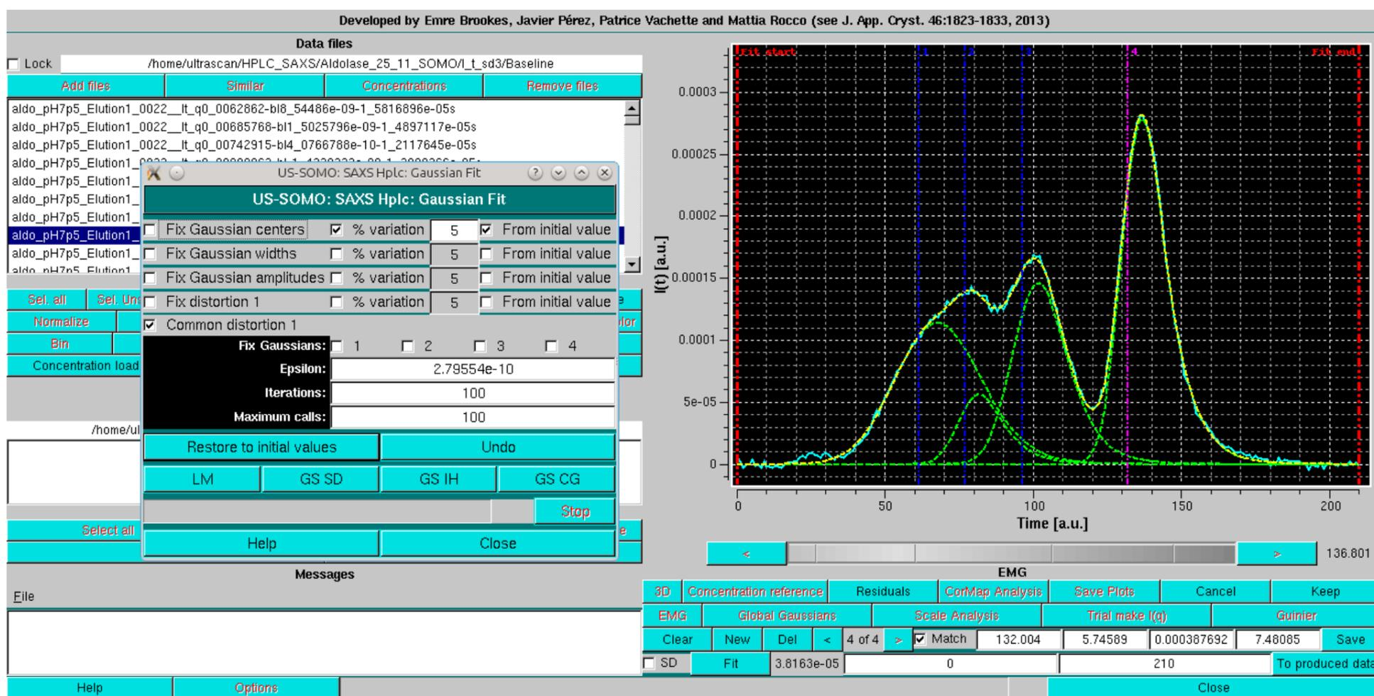
Bringing in the SD and releasing all constraints but the *Common distortion* produces a slightly improved fit:
