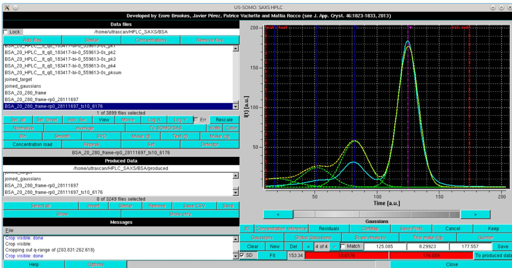
Pressing **Fit** will then bring up the **Fit** window (see [here](#)) and an initial round is done by keeping fixed both the position and widths. If necessary, a refinement can be done by keeping fixed the smallest, front eluting peak(s), and allowing only a limited shift to a % of the initial values from the widths and positions determined from the SAXS data (suggested: 2-3% max). This should compensate for slight misalignment between the concentration and SAXS detectors chromatograms.
