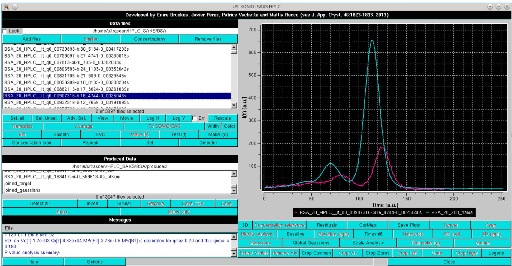
and pressing **Repeak** in the left-side command panel, which will bring up a small window asking to identify the target chromatogram (in case multiple were selected).
