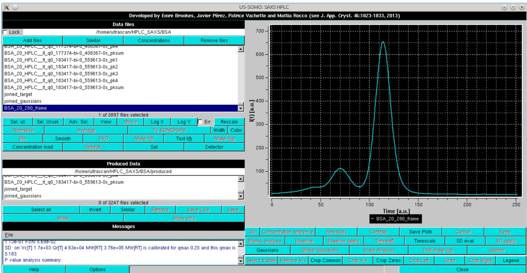
the first operation is to rescale it to one of the high intensity but relatively low-noise  $I(t)$  vs.  $t$  chromatograms. This is done by selecting the two files:
