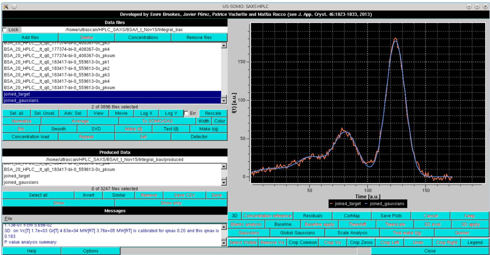
If available, a concentration chromatogram deriving from UV or refractive index monitors can now be processed. After uploading a suitable file with the *Concentration load* button:
