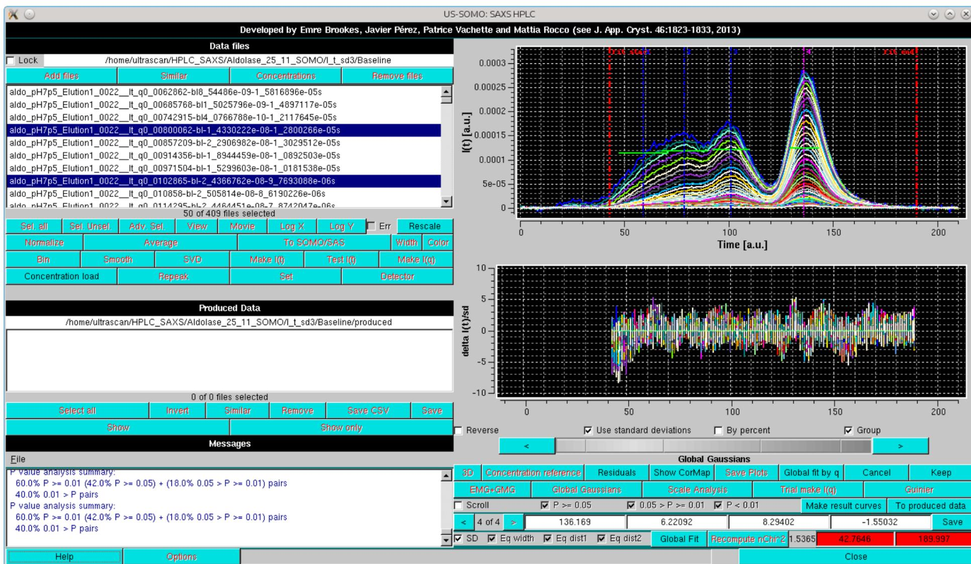
Here, already by looking at the *Residuals*, the fit appears to be improved, and the apparently larger residuals especially around the main peak are due to the very low SD associated with the data, amplifying the discrepancies. The goodness of the fit can be further checked by first restricting again the fit limits, then recomputing the residuals by pressing *Recompute  $n\chi^2$* , and subsequently pressing *Global fit by q*:
