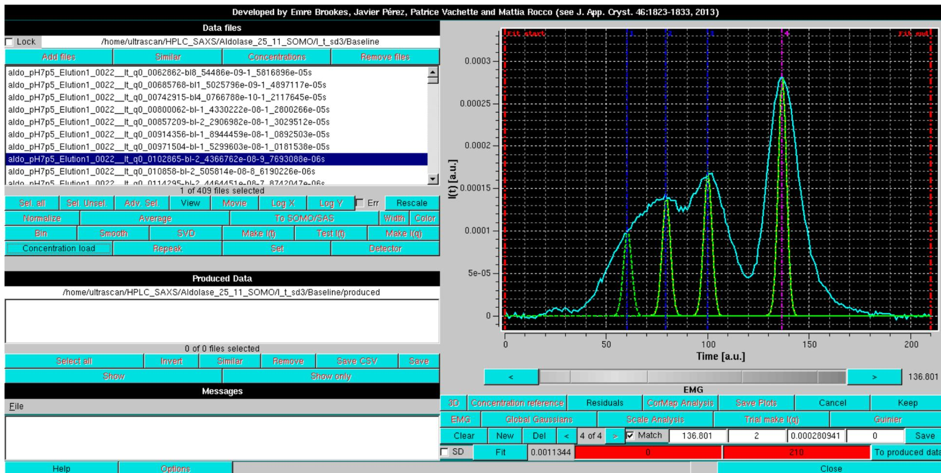
Note that four fields are now present in the third commands row. The first three are the center, width and amplitude of each Gaussian, as in normal Gaussian operation, while the fourth is the EMG Gaussian distortion (set to 0 at the beginning). All other commands are identical as for normal Gaussian operations. Once the initial set of EMG Gaussians is positioned, pressing *Fit* will bring up again the *Gaussian Fit* module:
