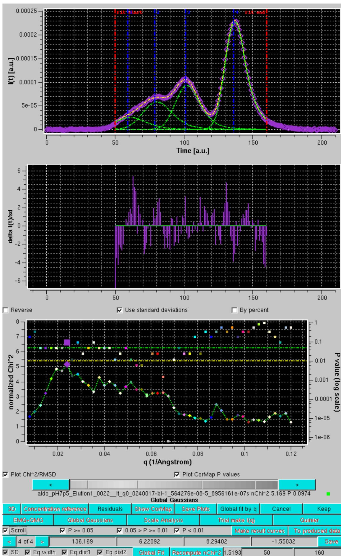
The current chromatograms pair is highlighted in both plots by an enlarged symbol (purple square in this case). Scrolling is performed by either using the grey-scale bar-wheel, or by clicking on the the "<" and ">" buttons placed at its sides. By selecting/deselecting the three checkboxes next to the *Scroll* checkbox ( $P \geq 0.05$ ,  $0.05 > P \geq 0.01$ ,  $P < 0.01$ ), only the subset(s) whose  $P$ -values are within those of the selected checkbox(es) will be scrolled.
